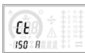
Press the ▲ key and dial Current Transformer primary current. Once the setting is done, press the
