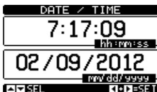
In this page, increase or decrease the numerical values with the ▲▼ keys. Use the ▶◀ keys to move from one number to the other. Confirm with the □ key.
