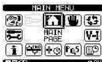
Select the desired menu with the **▲▼** keys and confirm with the **□** key. The selected menu is highlighted in reverse and at the centre a text description appears.
