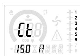
Press the ▲ key and dial Current Transformer primary current. Once the setting is done, press the
