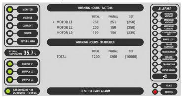
The SERVICE alarm is active when the number of working hours (PARTIAL) of either the motors or the unit exceeds the set value, indicated in brackets. In this situation, the relevant circle is red ant the card buzzer is active (but not the siren). Touch the SILENCER key to stop the card buzzer. The resetting of the alarm (and therefore the elimination of the red sign) is restricted to authorized Service Personnel by means of a password.
