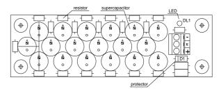
Any residual voltage can be easily detected by means of the LED mounted on the card: when the green LED is on, the capacitors are charged and voltage is available.
