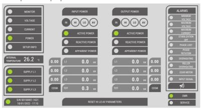
Select the desired power (active power [kW], reactive power [kvar], apparent power [kVA]) with the relevant key for input and output. The chosen option circle turns green and the indication below those key will be updated accordingly. Beside each phase power indication, the power factor relevant to that phase is also shown.
