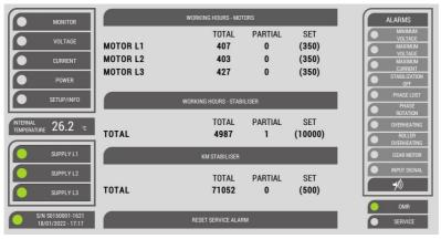
The **SERVICE** alarm is active when the number of working hours (**PARTIAL**) of either the motors or the voltage stabiliser exceeds the set value, indicated in brackets. In this situation, the relevant circle is red and the card buzzer is active (but not the siren). Touch the **SILENCER** key to stop the card buzzer. The resetting of the alarm (and therefore the elimination of the red sign) is restricted to authorized Service Personnel by means of a password.
