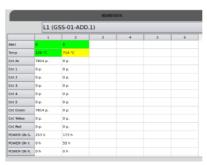
The temperature highlighted in yellow is the one that caused the anomaly. Touching the alarmed column, further information regarding the detected anomaly is displayed:
