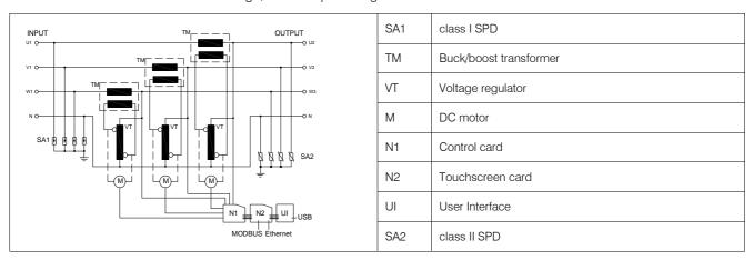
The remote communication is managed by the touchscreen card. Provided that the unit is connected to an Ethernet network, the interface screenshots can be reproduced remotely with a VNC software. The communication can also be established via a MODBUS® TCP/IP protocol (see the relevant chapter) in order to manage the information available.
